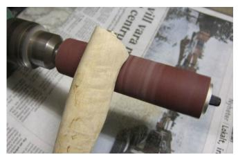
13 Shape the handle using a rotating sander and/or by hand. Starting from grit about 100 (European). Then approximately double the grit to 240, 400 and finer if you like. This handle is taken to 400 grit. The brass bolt is filed and sanded down.
